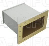
975WECAN Endlaunch Rectangular Waveguide to Coaxial Adapter 0.75-1.12GHz WR975 to N Type Female
