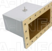
975WCAS Right Angle Rectangular Waveguide to Coaxial Adapter 0.75-1.12GHz WR975 to SMA Female
